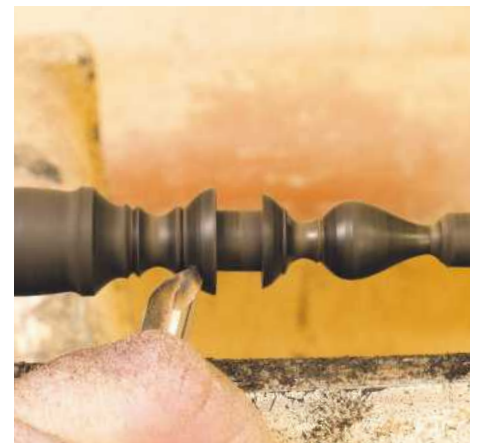
▲ Pic.27 The parallel section to the right of the tool is the spigot that will fit through the top. The tool he is using is the new 10mm Signature spindle gouge
